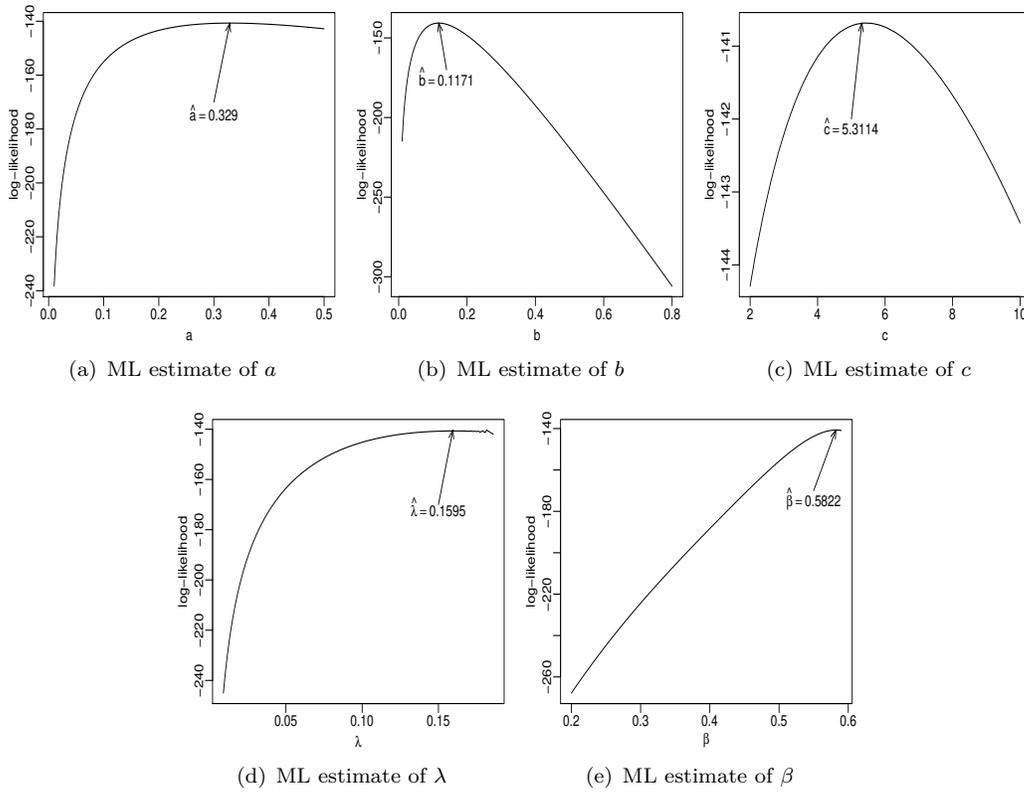
Figure 10. Profile log-likelihood functions for Kevlar/epoxy data.
